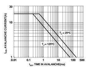
Figure 9. Unclamped Inductive Switching Capability
