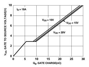
Figure 7. Gate Charge Characteristics
