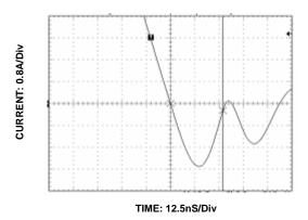
Figure 14. FDS8672S SyncFET Body Diode Reverse Recovery Characteristics
