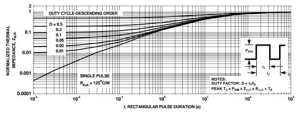
Figure 13. Transient Thermal Response Curve
