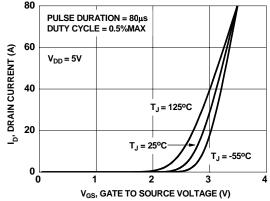
Figure 5. Transfer Characteristics
