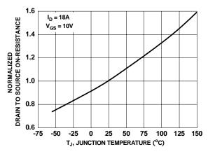
Figure 3. Normalized On-Resistance vs Junction Temperature
