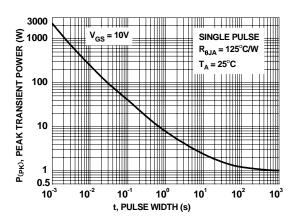
Figure 12. Single Pulse Maximum Power Dissipation
